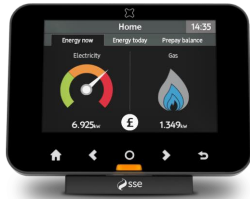
Figure 9b: Smart meter display monitor
