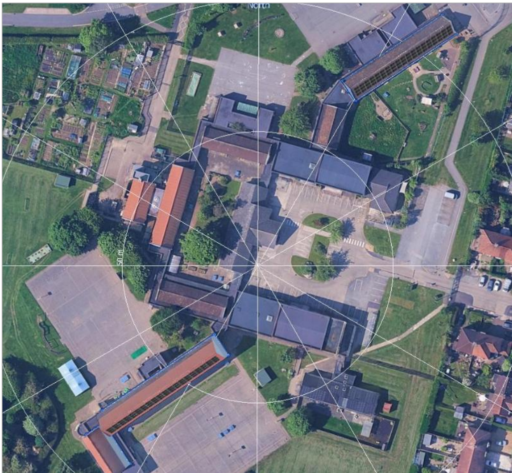
Figure 30 Proposed 70 kWp PV System
